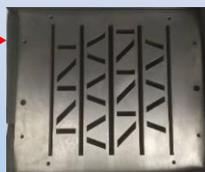
Multi-slit collimator based on Tungsten alloy
